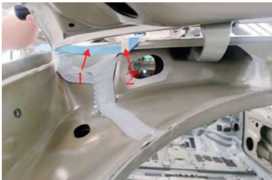
图3 黑车顶分界线胶带压紧工具压紧起始点示意图 Fig.3 Sketch map of startup site for press masking boundary tape at black roof
